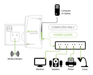
The LED monitoring light on the Embertec SmartSwitch™ PC will now light up for 3 seconds to indicate detection of connected equipment. This also indicates the Embertec SmartSwitch™ PC is monitoring your power consumption and providing power to the 'Power Saver' socket and then will switch off.
